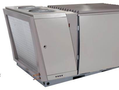
The Ice Bear unit creates and stores cooling energy at night by freezing water in an insulated storage tank. It cools during the day by circulating chilled refrigerant from that tank to the conventional air conditioning system, eliminating the need to run the energy-intensive compressor during peak daytime hours.
